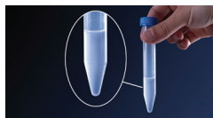
Figure 1: Before proceeding to step 4, ensure that the entire sample has been incubated and transferred to a fresh 15 mL centrifuge tube, as shown.
